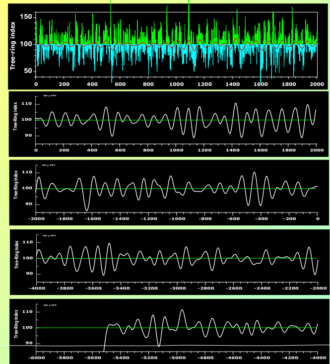
Fig.3. 50-yr FFT smoothing on the Finnish 7638-yr pine chronology brings the strong 84-yr cycle clearly visible.
